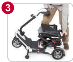
Fold and Lock Tiller
