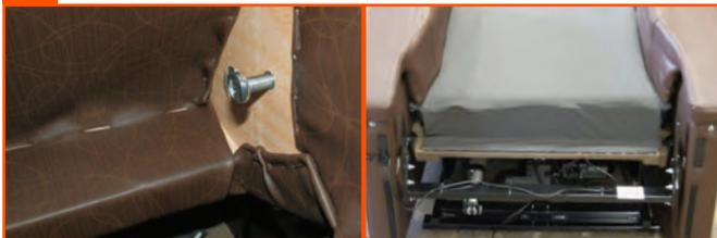
Remove backrest – remember to remove the screws securing the backrest brackets on the inside of the backrest
